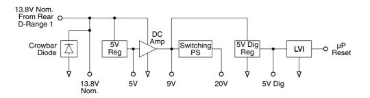
Figure 2.4 T835 Power Supply And Regulators Block Diagram
