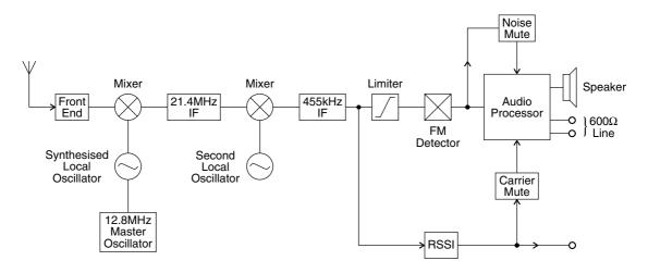
Figure 2.1 T835 High Level Block Diagram
