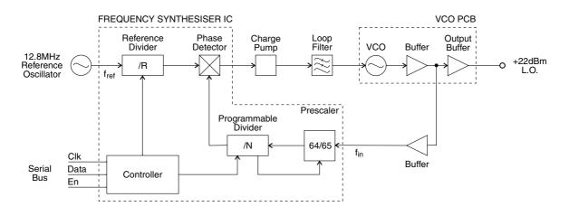
Figure 2.6 T835 Synthesiser Block Diagram
